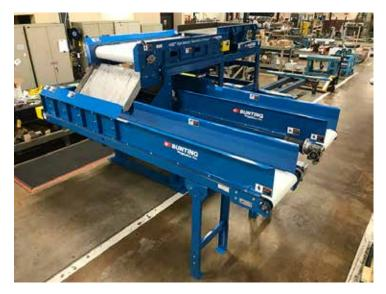
Note: Generally 2" minus fractions work great on 4"diameter HISC<sup>™</sup> Pulleys while larger 4"minus fractions need the 6" diameter HISC<sup>™</sup> Pulleys.
